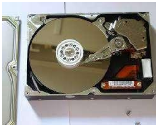
Hard drive showing magnetic platters
