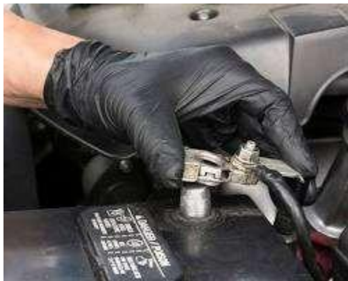
Cleaning battery terminals
