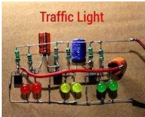
Traffic light circuit board with capacitors
